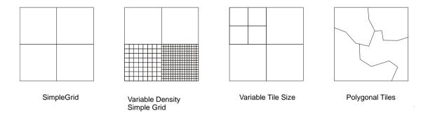
Figure 8-19 - Tiling Scheme Types
