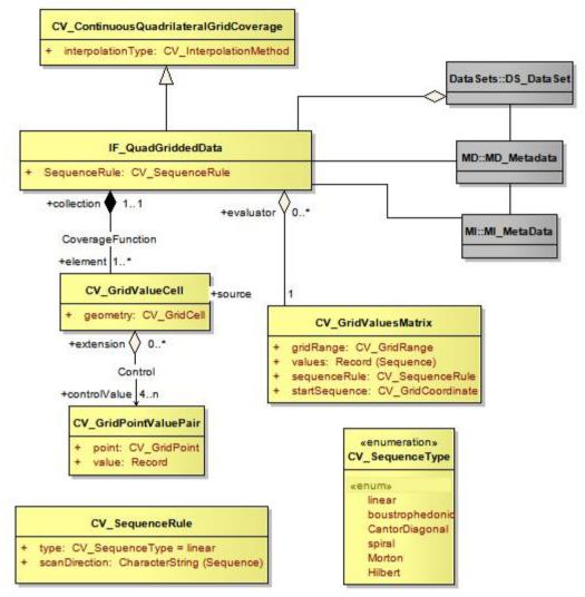
Figure 8-28 - Template Application Schema for a Quadrilateral Grid Coverage
