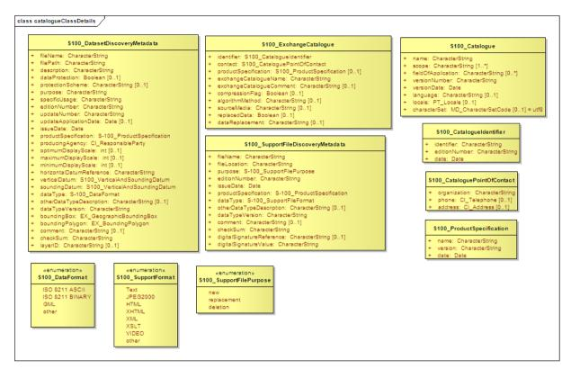
Figure 4a-D4 S-100 Exchange Set - class details
