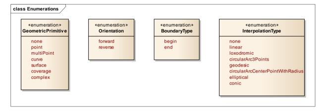
Figure 9-4 — Input Schema Enumerations
