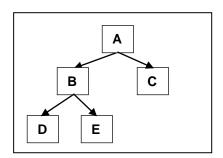
Where A is the root node and parent of node B and node C. Node B is the root of a sub-tree and the parent of nodes D and E.
