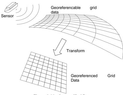
Figure 8-26 - Georectified Data
