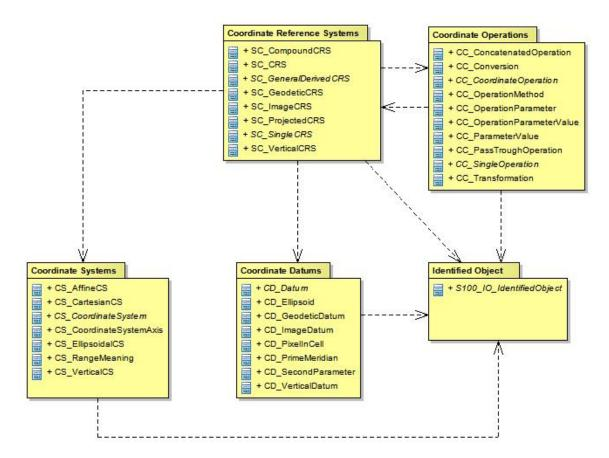
Figure 1-15 — Example package structure
