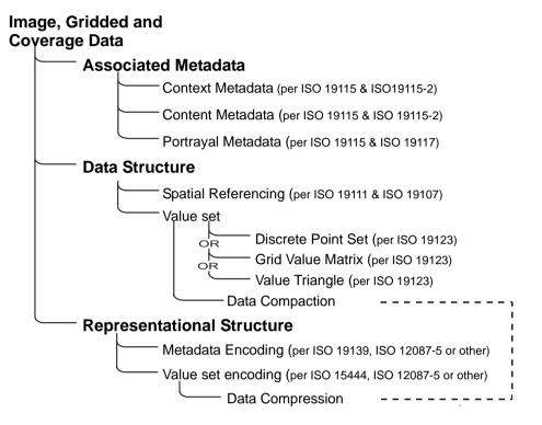
Figure 8-3 - Image and Gridded Data Structure
