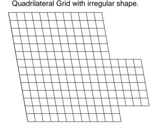
Figure 8-8 - Quadrilateral Grid with Outset
