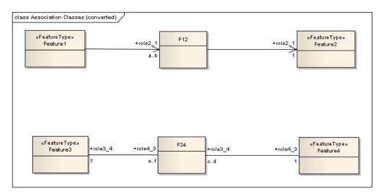
Figure 10b-3 – Model after conversion of association classes (from OGC 10-129r1 / ISO/DIS 19136-2)
