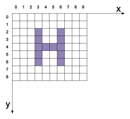
The graphic above shows a simple pixmap with width 10 pixel and height 9 pixel. Most of the pixels are transparent (here white) some pixels are coloured.
