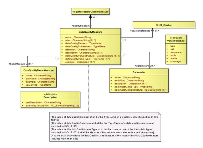
Figure 4c-A2 — Data Quality Measure Registry UML (from ISO 19138)
