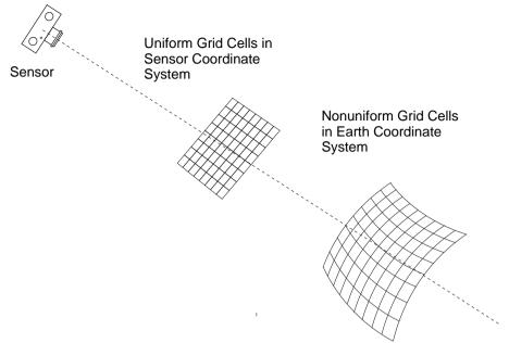
Figure 8-25 - Non Uniform Spacing of Grid Cells
