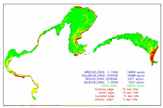
Figure II-2 - The analyzed chart of ice thickness and edge of the Bohai Sea on 11 February 2005
